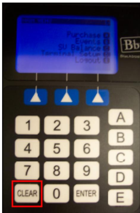
This is the Main Menu. From here you can select the particular screen you need in order to perform the correct action. When ever you are on a different screen and need to return to the Main Menu, press the **Clear** button. This will always return you to the Main Menu.
