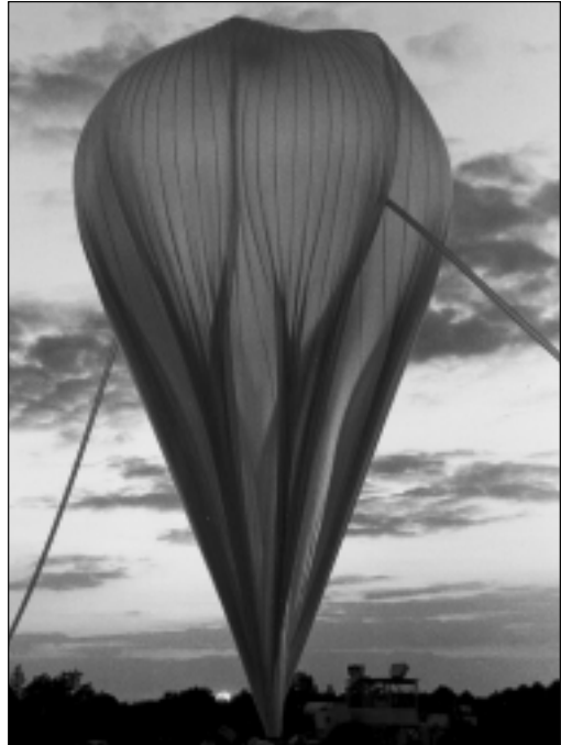
Final inflation of an instrument-carrying helium balloon before launch from Palestine, TX
