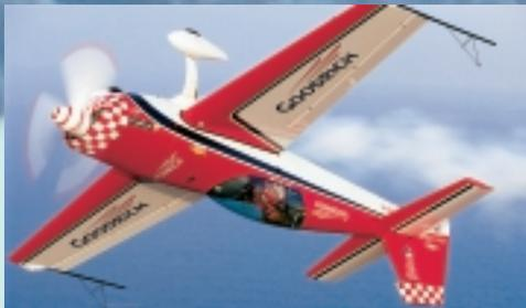
Here's an uplifting explanation. A wing is shaped and tilted so air moves faster over the wing than under it. This creates an upward force called lift. A wing will produce lift even while flying upside down, as long as the wing's front edge is tilted far enough above its rear edge.
