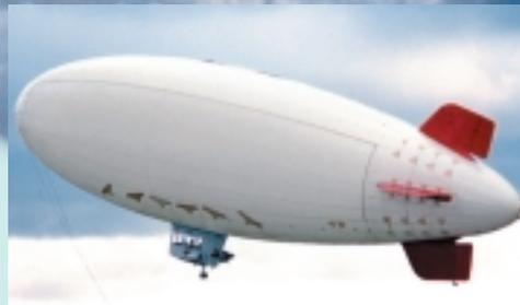
A blimp will take you pretty far up, but not above the atmosphere. The reason is buoyancy, the upward force of the air. Buoyancy is created by the difference in air pressure between the bottom and top of the blimp. It decreases the higher you go. The blimp stops rising when its buoyancy equals its weight.
