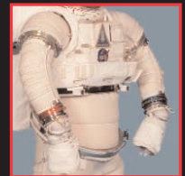
With the outer suit fabric removed, bearings for mobility are visible at the shoulders, wrists, and waist. The astronaut enters the suit by pulling on the lower torso (ganth), slipping into the upper torso, and snapping the waist bearing rings together.
