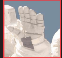
When pressurized, spacesuits become stiff. Suit gloves need many joints to permit finger dexterity. A small wrist mirror permits reading control settings on the front of the suit.
