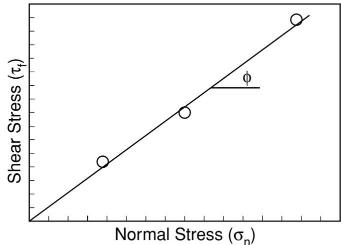
Figure 7. Coulomb shear stress versus normal stress relation.
