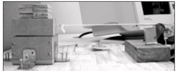
Figure 12. An assembled DST box, ready to slide.
