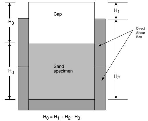
Figure 11. Determining the height of the sand specimen.
