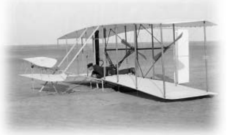
Wilbur in the damaged flyer after his unsuccessful trial on December 14, 1903. His hand still grips the wooden control lever.
